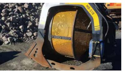
At Flommen nature reserve, attempts were made using a built-in rotating drum to sift away the Japanese rose and its roots from the sand directly in the bucket. The method worked well except the bearings became full of sand and needed to be replaced at regular intervals, which meant that it stood still so much that we had to abandon the method.
